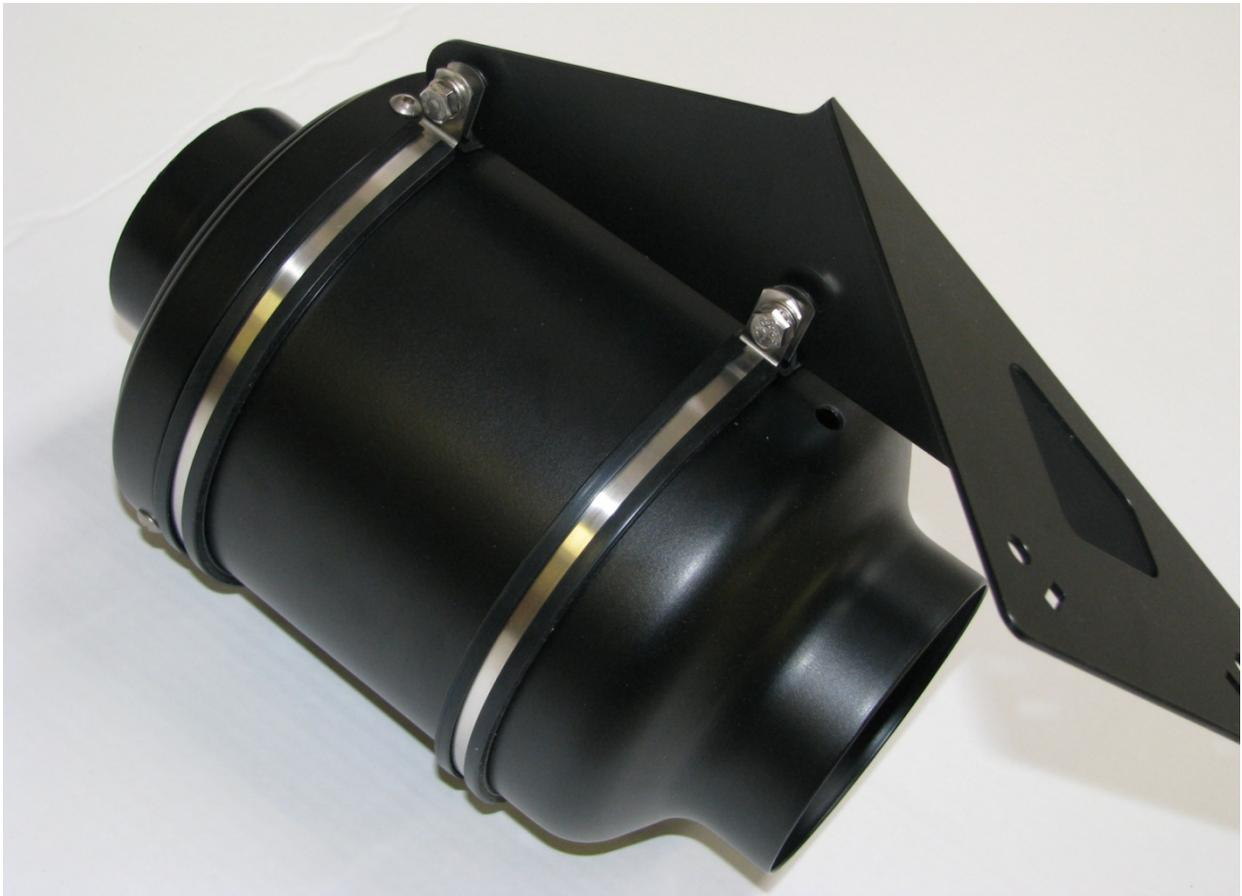
Fit the bracket and the retaining straps to the airbox as shown ensuring the bracket lines up with the water drain hole and lid retaining screw (opposite side to the ITG sticker).
