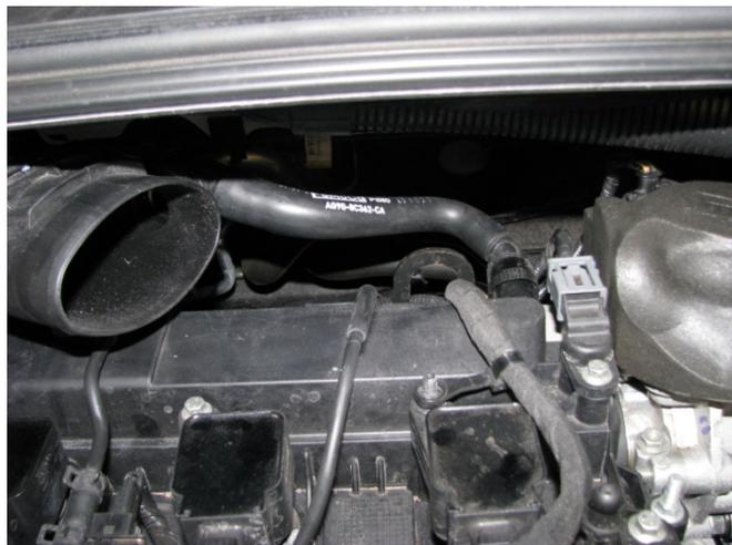
With the breather pipe out of the way, you should now have enough room to get down the back of the engine and disconnect the crossover pipe from the turbo.
