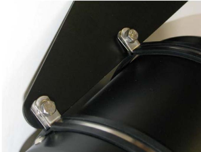
Leave these bolts as loose as possible as you will need to make a few adjustments later as even when loose, the straps will grip quite well. It will also help to align the duct as shown below and tighten up the hose clip.
