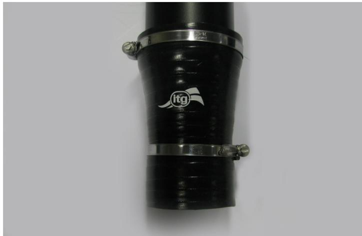
Now, thread the crossover pipe down the back of the engine and push the silicon hose down onto the turbo as firmly as possible until it bottoms out on the step in the hose. With the pipe in place, connect the breather hose and then tighten the clamps, then slacken off the clamp on the turbo hose, drop it down into place and fully tighten the turbo connection.
