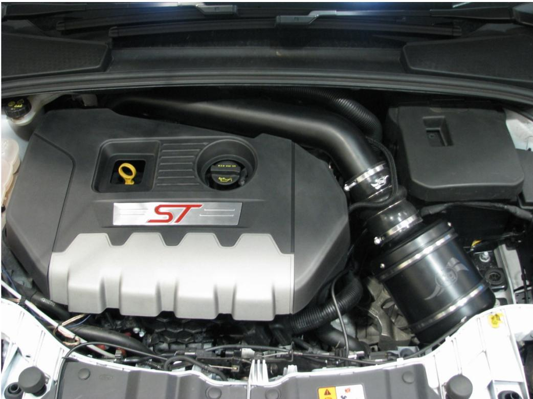
When you are happy with the position of airbox all that is left to do is fit the silicon hose, this will collapse down enough for you to squeeze it into place with the airbox fitted. You will need to completely unwind the hose clips to fit them into position, and then fully tighten the clips once in place.
