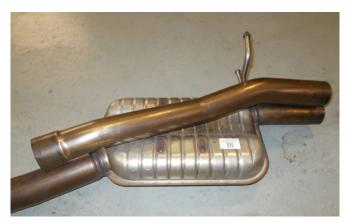
Remove the original system, place the resonator delete pipe over the top of the system.
