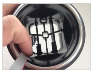
Insert VIDI cable between outer housing wall and far upright as shown.
